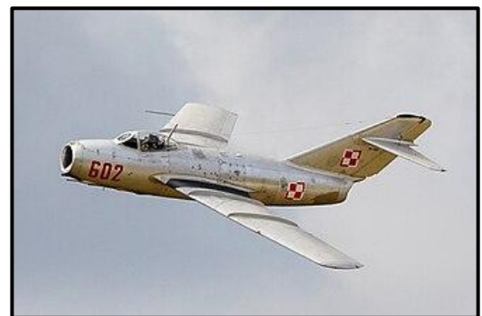
The Soviet MiG-15 was one of the first successful swept-wing fighters.
